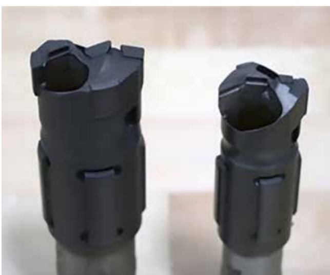
Brazed BTA heads - carbide inserts and guide pads are brazed onto the drill head
