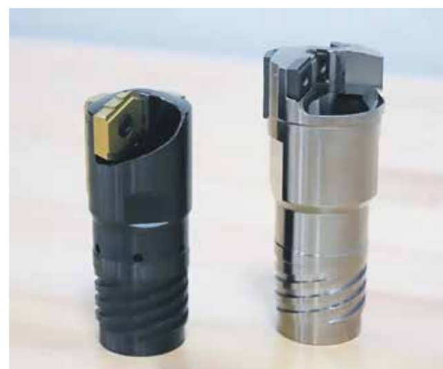
Indexable BTA heads, with inserts mounted directly to the head
