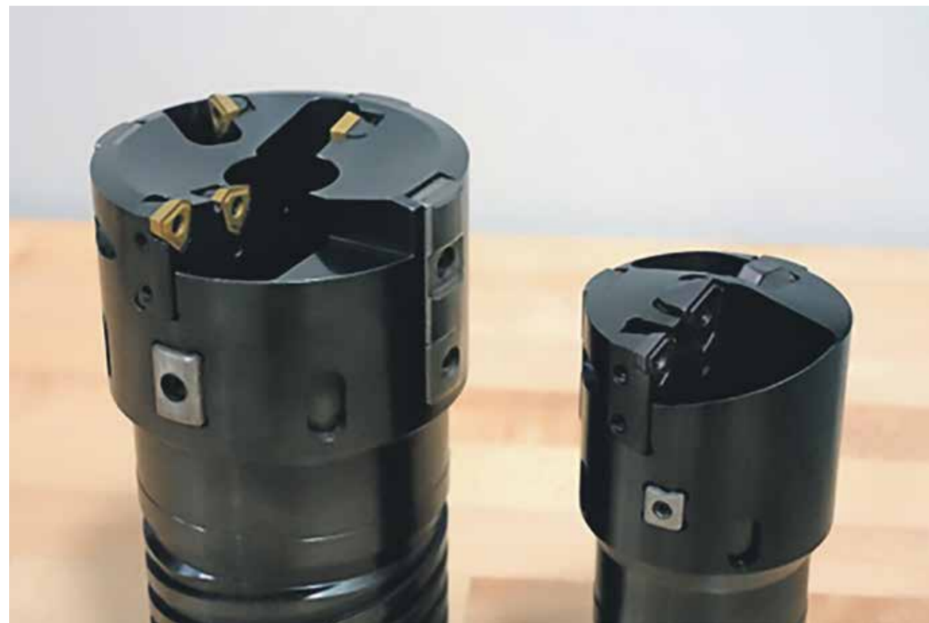
BTA drilling heads with cartridge-mounted indexable inserts.
