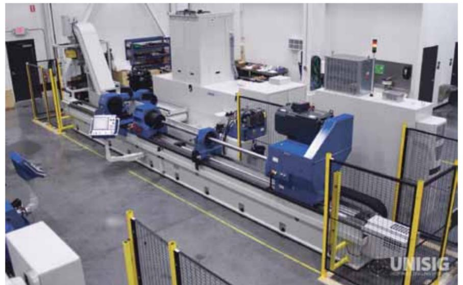
workpieces, and this is where UNISIG's USC-TS series can help. Using multiple spindle configurations and programmable positioning, UNISIG's machines bring confident drilling to heat exchanger tube sheets.
