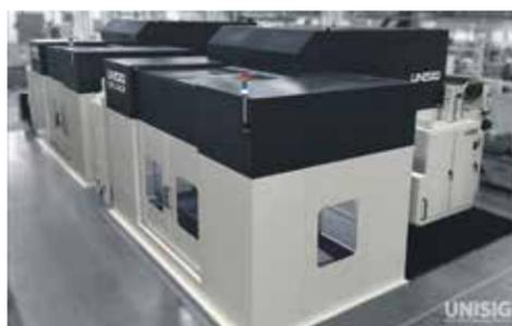
UNISIG has standard models which can drill holes of less than 1 mm diameter in titanium medical components, while on the other end of the spectrum they can build machines that drill holes which are 500 mm in diameter and over 10 m deep in huge high strength forgings.
