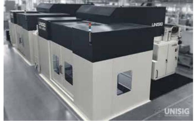
require thousands of precision holes in large and high-value workpieces, and this is where UNISIG's USC-TS series can help. Using multiple spindle configurations and programmable positioning, UNISIG's machines bring confident drilling to heat exchanger tube sheets.
