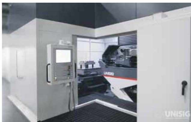
tools; modular fixturing to reduce setup and allow for process planning; and dual pallet loaders to allow for automatic workpiece exchange, improving machine utilisation and unattended machining.
