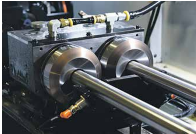
At DRG Manufacturing, a dual-spindle UNISIG UNE12-2 gundrilling machine, with 12mm maximum part diameter, drills barrels for the shop's automated operations
