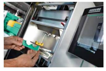
component layer-by-layer from a 3D model dataset. This technology can be used to integrate complex functions into a component, as well as producing more intricate geometries that cannot be achieved using conventional injection moulding. Droplet generation and discharge is central to the process, requiring
