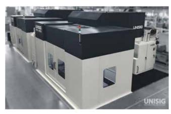
require thousands of precision holes in large and high-value workpieces, and this is where UNISIG's USC-TS series can help. Using multiple spindle configurations and programmable positioning, UNISIG's machines bring confident drilling to heat exchanger tube sheets.
