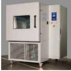
engineers designed an innovative CO<sub>2</sub> cascade system, capable of achieving a range of +80/ -40c at high rates of temperature change. As an inert gas, CO<sub>2</sub> has a major advantage in this application over alternative refrigerants which are either highly flammable, less efficient or have a far higher GWP (Global Warming Potential)
