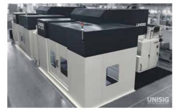
require thousands of precision holes in large and high-value workpieces, and this is where UNISIC's USC-TS series can help. Using multiple spindle configurations and programmable positioning, UNISIC's machines bring confident drilling to heat exchanger tube sheets.
